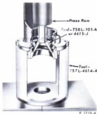
FIG. 23—Removing Pinion Rear Bearing Cup
