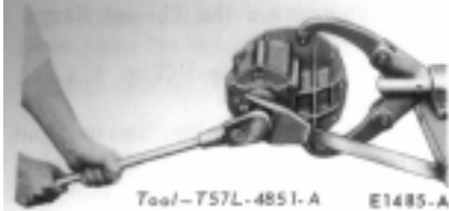
FIG. 16—Removing Pinion Shaft Lock Nut
