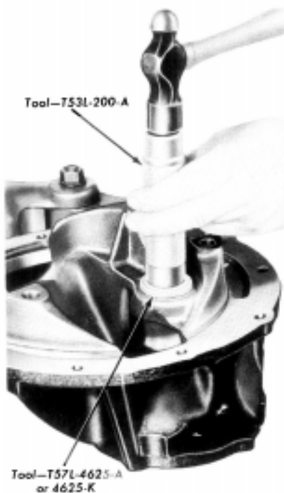
FIG. 20—Removing Pilot Bearing
