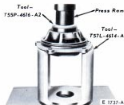
FIG. 25—Installing Pinion Rear Bearing
